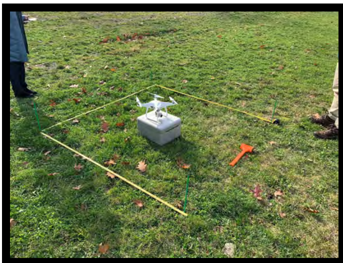
Figure 6. DJI Phantom 4 Drone used for large scale snow depth measurement
